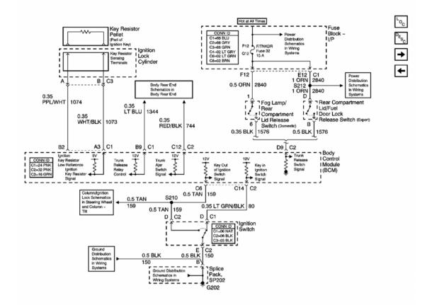
**Fig. 3: Ignition Key Signals and Trunk Release Switch Signal Schematic Courtesy of GENERAL MOTORS CORP.**
