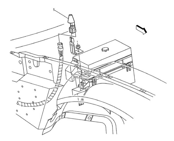
**Fig. 6: Hood Ajar Switch Component View Courtesy of GENERAL MOTORS CORP.**
