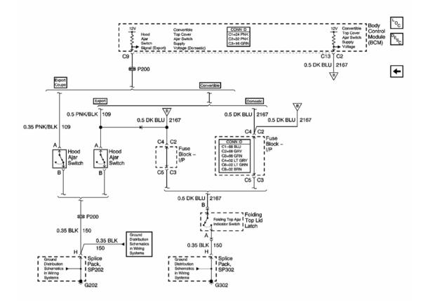
Fig. 4: Hood Ajar Switch Signal and Convertible Top Cover Ajar Switch Supply Voltage Schematic Courtesy of GENERAL MOTORS CORP.
