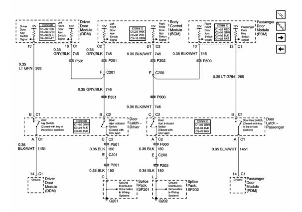
**Fig. 2: Door Signals Schematic** Courtesy of GENERAL MOTORS CORP.
