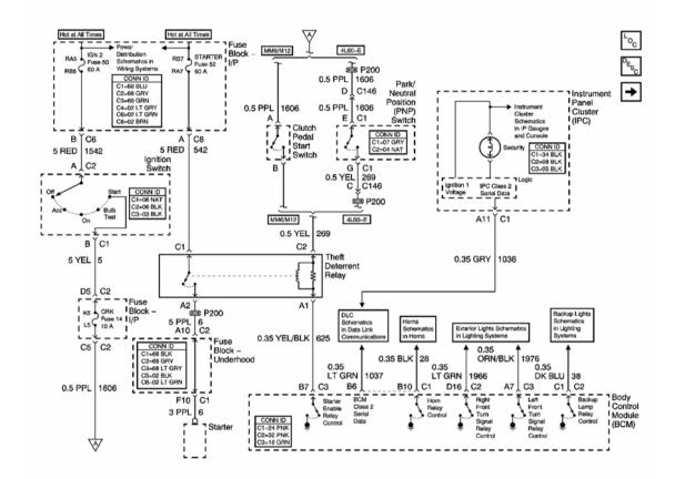
Fig. 1: Theft Deterrent Relay, Security Indicator, Lighting and Horn References Schematic Courtesy of GENERAL MOTORS CORP.
